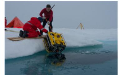
The ROV is lowered into a melt pond. In the background the „operation center“ tent is visible, as well as the tripod holding the reference sensor (Photo: S. Hendricks)
