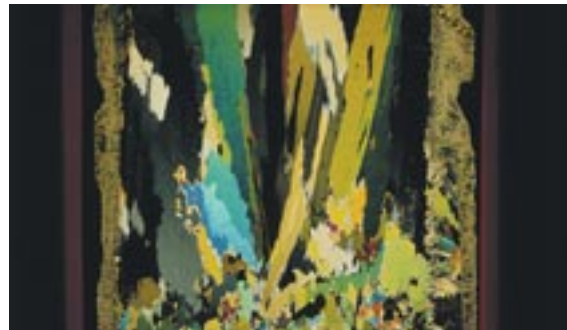
▲ Thin section of an ice sample
