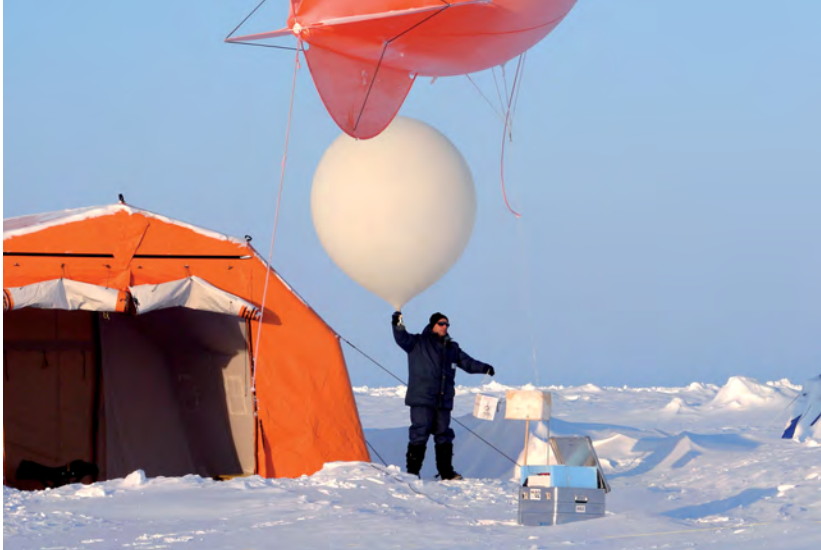
◀ Expedition to the Arctic: start of an ozone probe on ice floe NP-35, in the foreground a red tethered balloon. (photo: J. Graeser)
