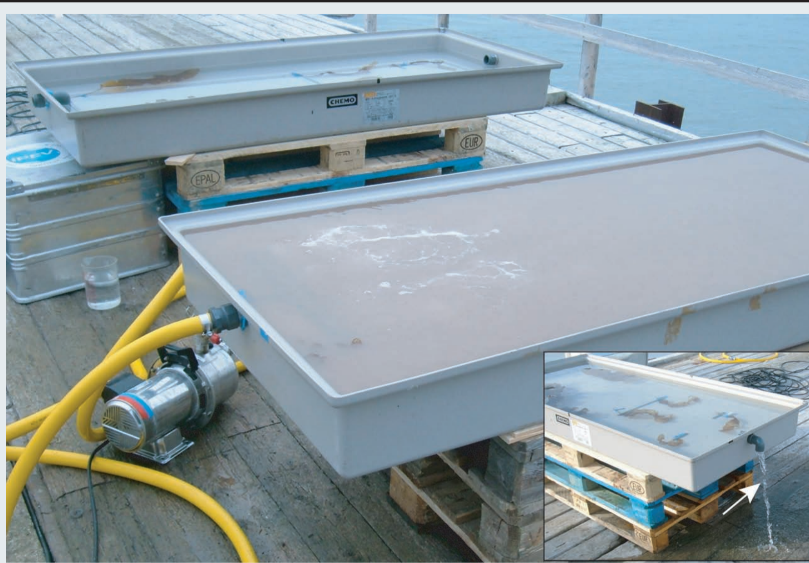
Outdoor tank experiments with marine macroalgae ( Saccharina latissima ); sediment-free (rear); sediment-laden (front)
