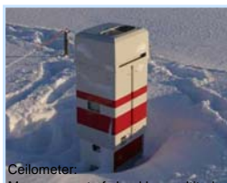
Ceilometer: Measurement of cloud base altitude.
